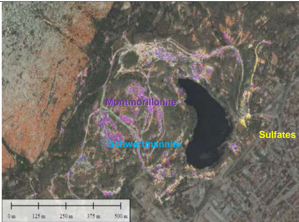
Water-expanding clays (e.g. montmorillonite) which may results in landslide hazards propagation and potential pitwall rupture
